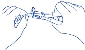
Place sealing clip onto folded tubing
